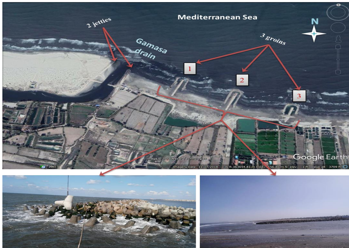
Figure 2. Protection structures at Gamasa drain exit (groins and jetties) (Google earth maps).
