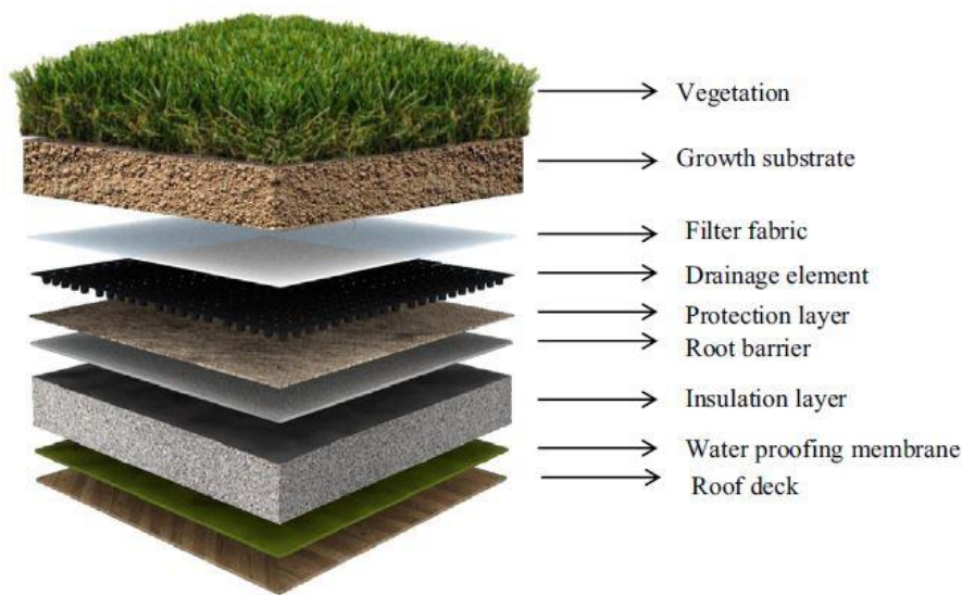
Fig. 1: Cross-section of a typical green roof. Source: Vijayaraghavan (2016)
