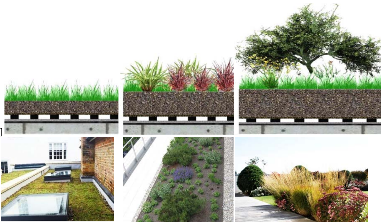
Fig. 2: Extensive (left), semi-intensive (middle) and intensive (right) green roofs. Source: (Besir & Cuce, 2018; http://www.greenroofers.co.uk/green-roofs/ )
